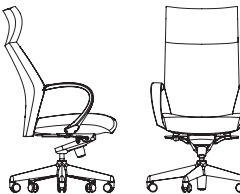
9875 High Back, Fully Upholstered Border Back, Arc Arm Fully Upholstered W 24-27.5" D 18" H 43.5-46" SH 16.75-21" AH 24.5-27.5"
